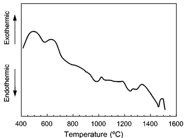
Figure 1 DTA diagram of the cordierite precursor oxides (raw materials) mixture, at a heating rate of 15 °C min<sup>-1</sup>.
