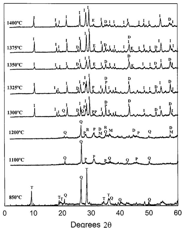
Figure 2 X-ray diffraction patterns of cordierite precursor honeycomb after calcination at different temperatures. (T: talc, Q: quartz, P: protoenstatite, R: cristobalite, M: mullite, D: corundum, E: spinel and I: hexagonal cordierite or indialite).
